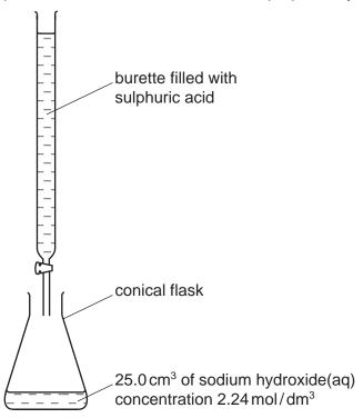
(a) 25.0 cm³ of aqueous sodium hydroxide is pipetted into a conical flask.
