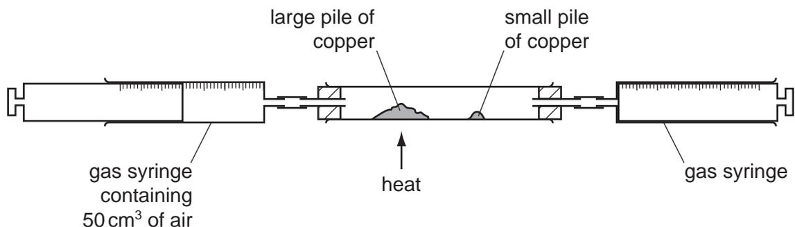
The gas syringe contains 50 cm<sup>3</sup> of air. The large pile of copper is heated and the air is passed from one gas syringe to the other over the hot copper. The large pile of copper turns black. The gas is allowed to cool and its volume measured.
