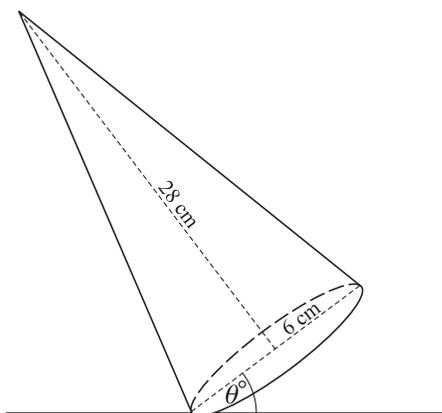
A uniform solid cone has vertical height 28 cm and base radius 6 cm. The cone is held with a point of the circumference of its base in contact with a horizontal table, and with the base making an angle of  $\theta^\circ$  with the horizontal (see diagram). When the cone is released, it moves towards the equilibrium position in which its base is in contact with the table. Show that  $\theta < 40.6$ , correct to 1 decimal place.
