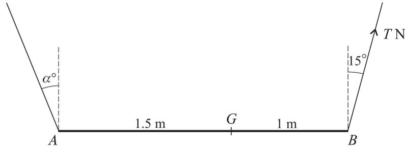
A non-uniform rod  $AB$  of length 2.5 m and mass 3 kg has its centre of mass at the point  $G$  of the rod, where  $AG = 1.5$  m. The rod hangs horizontally, in equilibrium, from strings attached at  $A$  and  $B$ . The strings at  $A$  and  $B$  make angles with the vertical of  $\alpha^\circ$  and  $15^\circ$  respectively. The tension in the string at  $B$  is  $T$  N (see diagram). Find
